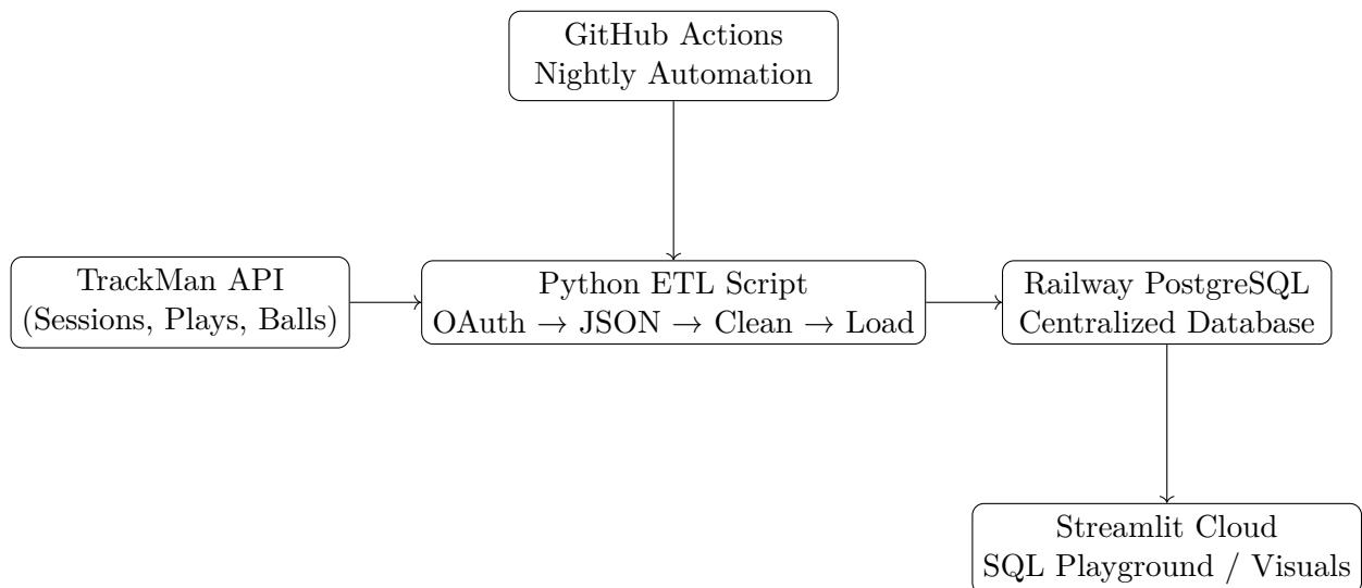
This flowchart illustrates the full TrackMan ETL architecture. Data flow proceeds from left to right: the TrackMan API provides raw pitch- and session-level data, the Python ETL script authenticates, cleans, and loads the data into Railway's PostgreSQL database, and
